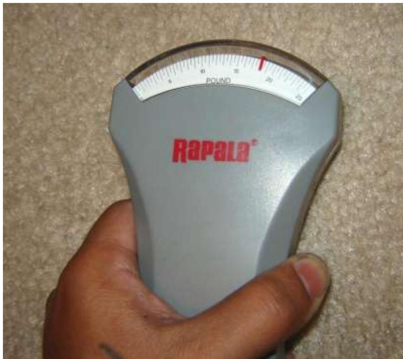
For a 1911 commander model, the compression point where you take the reading from is 1.125".
