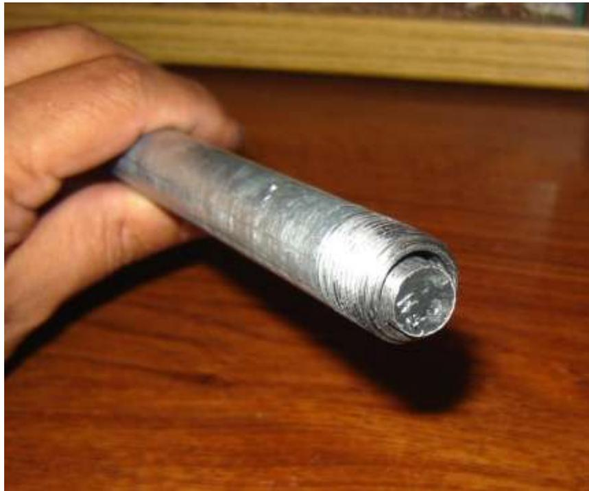
After the bolt head (and threads) are ground down, the next step is to get a few washers and stack them onto the end of the pipe nipple. (In this picture I only show 2 washers, but in the end I had to use 4 of them, add more later).
