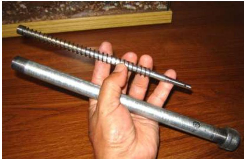
Once the spring is placed onto the hex bolt, insert both of them into the pipe nipple as shown in the next picture.
