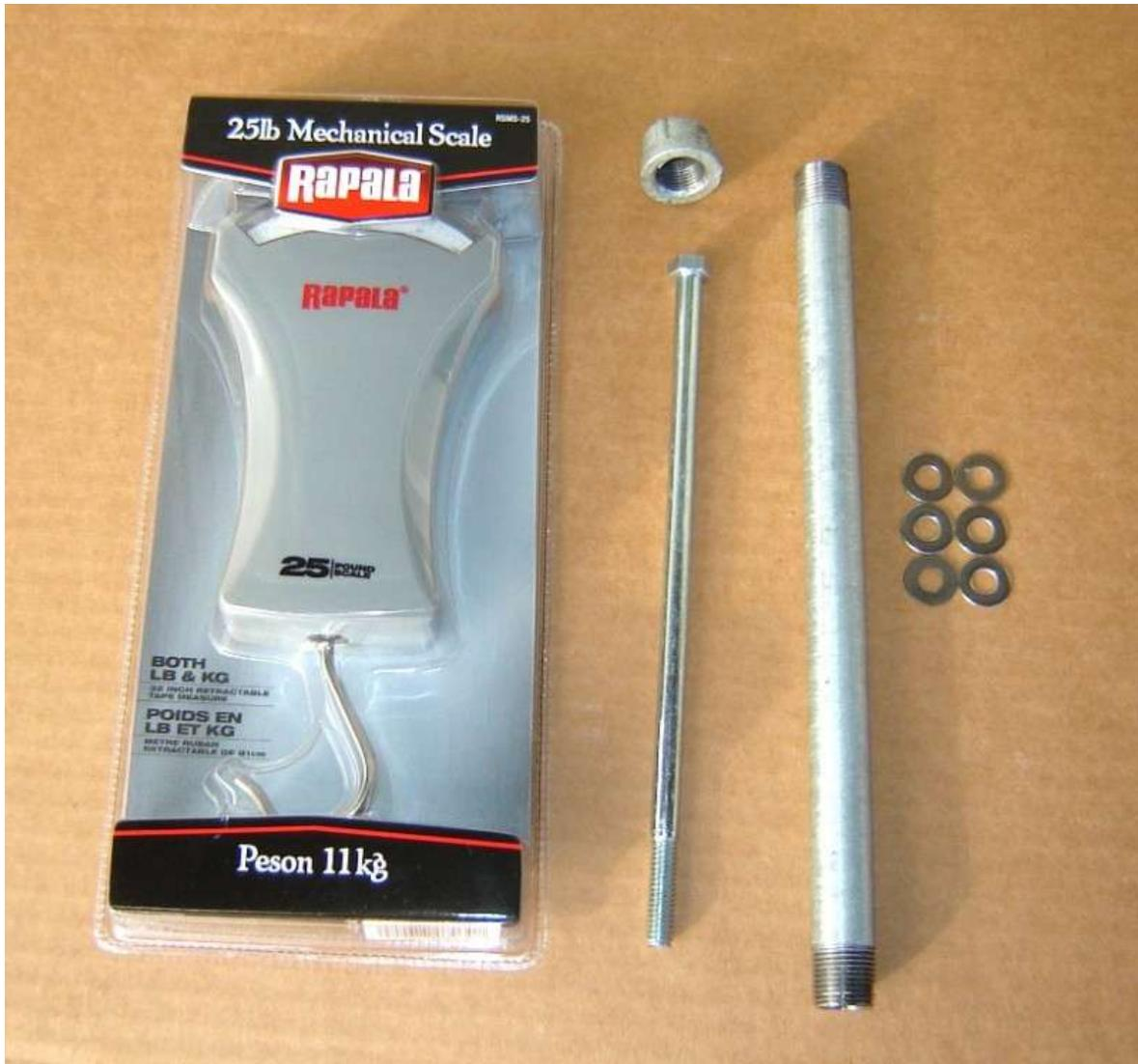
Below are a few pictures of the new bolt and the pipe nipple. The bolt head will need to be ground-down to fit inside the pipe nipple. Here are a few pictures to show you a before and after of the bolt head and threads.
