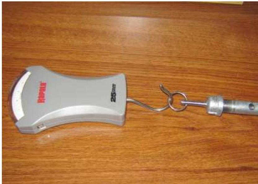
Pull the gauge against the scale until bolt head reaches the window at the 1.625" mark, this is the correct compression of the spring. When the top of the spring/bolt head reaches the mark on the "window," the recoil spring is compressed to the specified 1.625" point, and the poundage on the scale is read.
