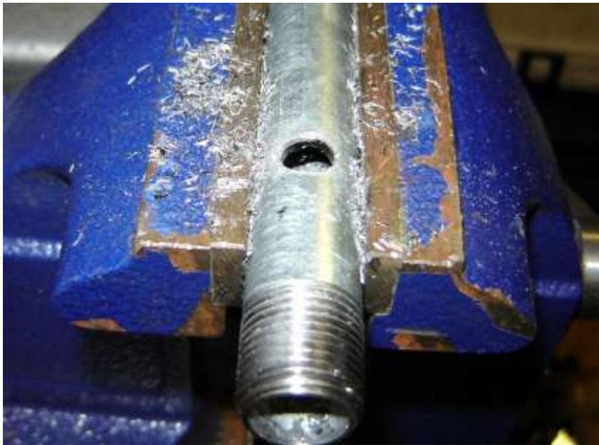
Drilled a small hole in the threaded end of the hex bolt.
