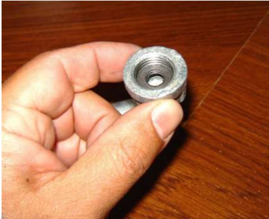
Now we take an important measurement. This measurement will be taken from the end of the pipe nipple where the cap was removed from. For a 1911 pistol (Government model), the spring must be compressed to a size of 1.625" inches when taking the measurement for the spring poundage, (As per a note found on the Brownell's website, and also another pretty good source "Wolf Springs" also supports this).
