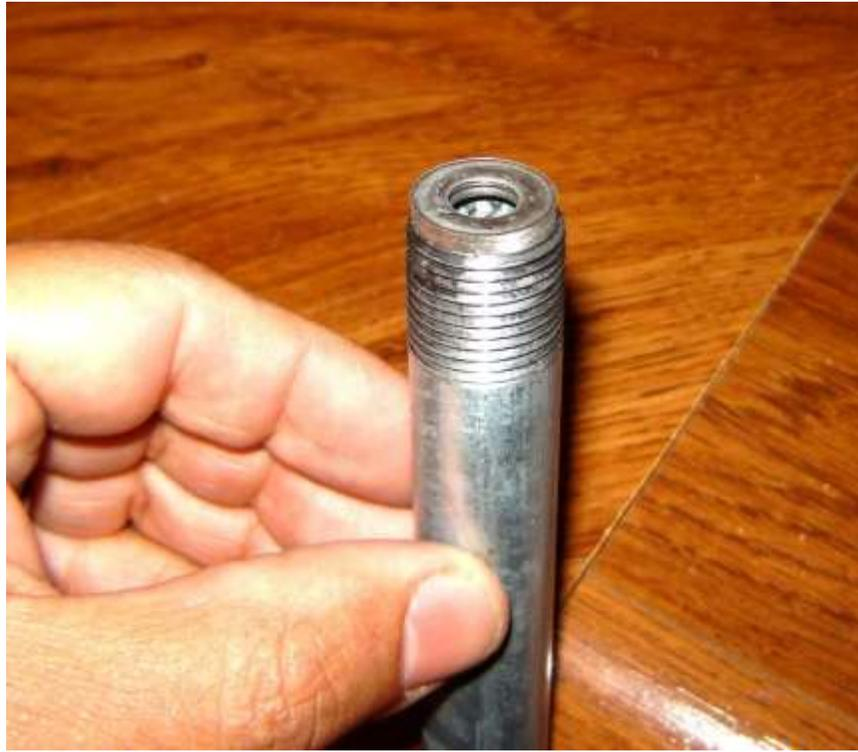
After the washers are stacked on the end of the pipe nipple, get the cap and screw it on very tightly to seat the washers onto the end of the pipe nipple. This is a very important step, as the washers must be flush with the bottom of the pipe nipple.
