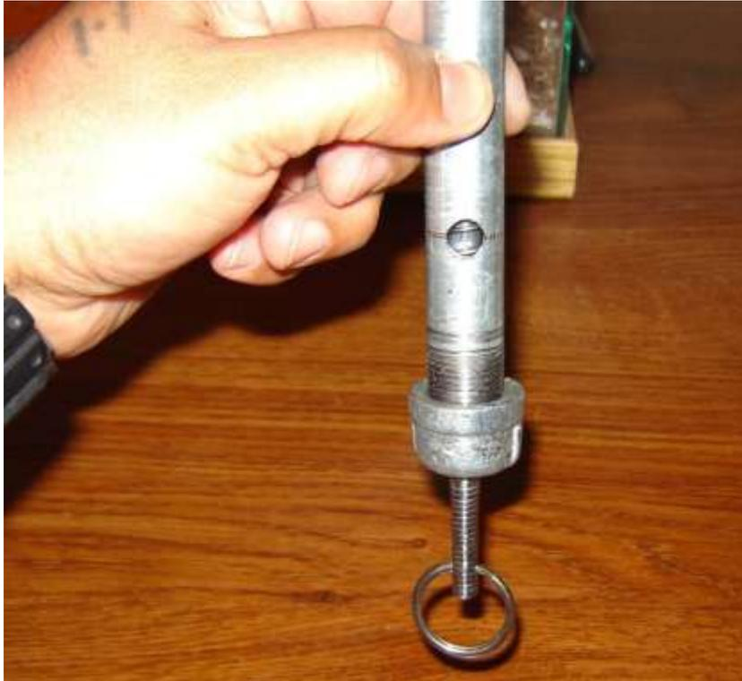
Now just hook-up the ring to the fish weighing scale and we're ready to check the spring.
