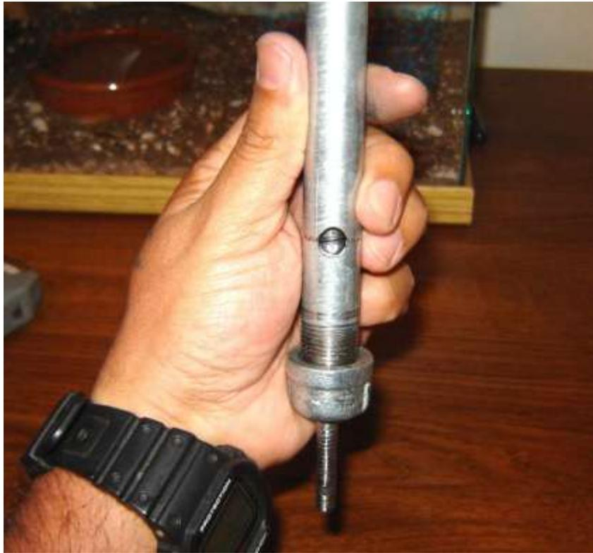
Once the parts are in the pipe nipple, place a heavy duty ring into the small hole drilled onto the threaded portion of the hex bolt. Also note of the line engraved into the sides of the "window". This is the center line of the window, which is EXACTLY 1.625" inches. When the bolt head and spring reach this line, we need to stop and take our reading.
